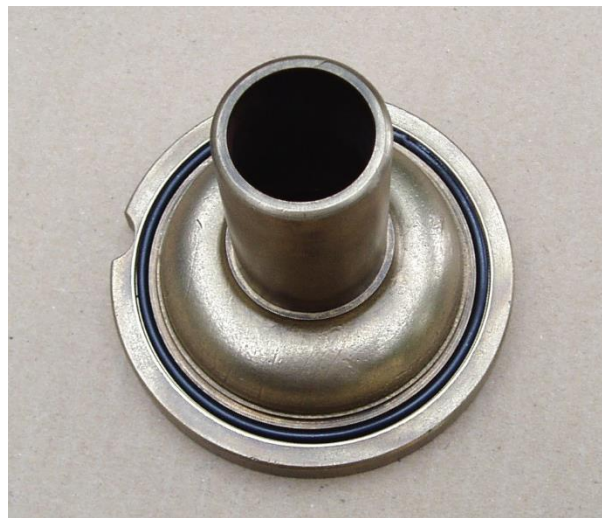
Figure 5. Illustrates the 'O' ring installed in groove.
